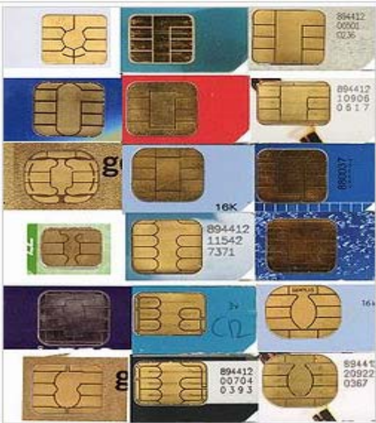
Many different pad layouts can be found on a contact Smart card
